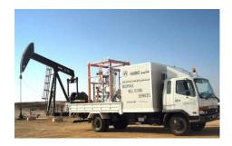
Haimo's **Low Production Tester**–LPT is developed primarily to address accurate measurement of low flowing and slugging wells.
